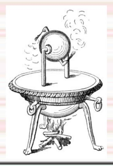
The first steam engine was created in 1<sup>st</sup> century AD by the Hero of Alexandria and was know as a aeolipile. But after that forgotten until 1680 when Denis Papin built a steam powered device.
