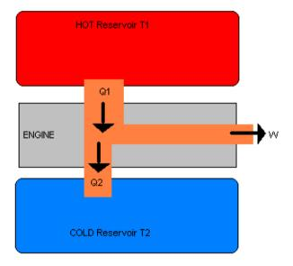
A heat engine is a device that converts heat to usable energy.
