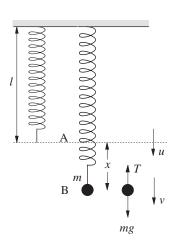
Consider the question for any mass m displaced a distance l+x from the level at which the spring is suspended. Here l is the natural length of the spring.
