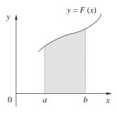
If a variable force F(x) moves a body of mass m from x = a to x = b then Newton's law of motion gives
