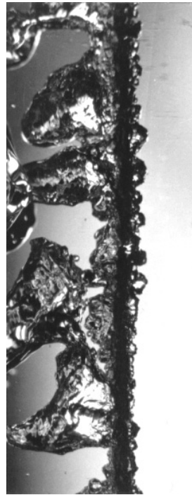
3.75 cm length of 0.164 cm diam. wire in benzene at earth-normal gravity, q=0.35 \times 10^6 \text{ W/m}^2 c. Two views of the regime of slugs and columns.
