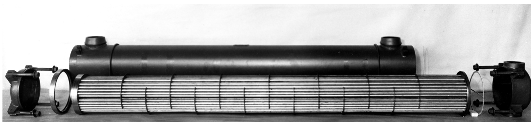
Figure 3.5 Typical commercial one-shell-pass, two-tube-pass heat exchangers.
