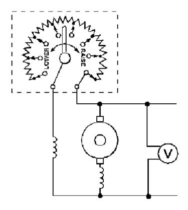
Figure 1-21.—Hand-operated field rheostat.
