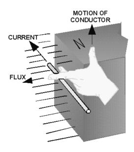
AN **ELEMENTARY GENERATOR** consists of a single coil rotated in a magnetic field. It produces an ac voltage.
