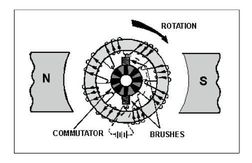
THE DRUM-WOUND ARMATURE consists of coils actually wound around the armature core so that all coil surfaces are exposed to the magnetic field. Nearly all dc motors have drum-wound armatures.
