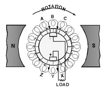
Figure 1-7.—Commutation of a dc generator.
