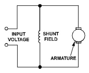
Figure 2-4.—Shunt-wound dc motor.
