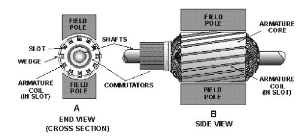
**MOTOR REVERSAL** in a dc motor can be accomplished by reversing the field connections or by reversing the armature connections. If both are reversed, rotation will continue in the original direction.
