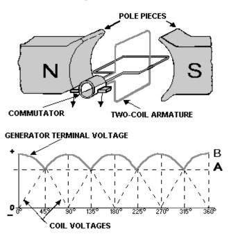
Figure 1-5.—Effects of additional coils.
