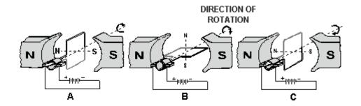
**COUNTER-ELECTROMOTIVE FORCE** is generated in a dc motor as armature coils cut the field flux. This emf opposes the applied voltage, and limits the flow of armature current.
