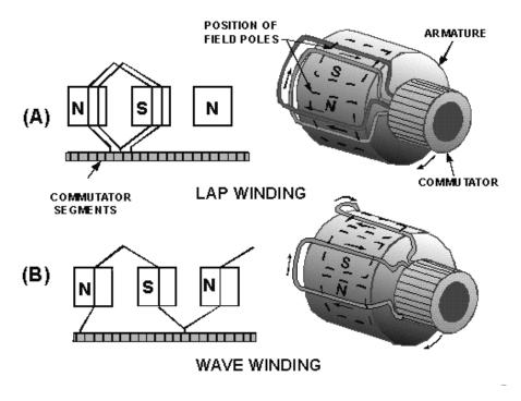
Figure 1-14.—Types of windings used on drum-type armatures.
