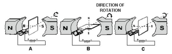
Figure 2-2.—Dc motor armature rotation.
