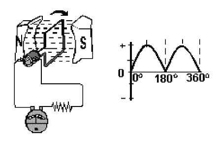
A MULTIPLE COIL ARMATURE (adding coils to the armature) decreases the ripple voltage in the output of a dc generator, and increases the output voltage.
