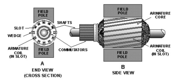
Figure 2-7.—Drum-type armature.
