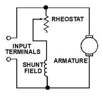
Figure 2-8.—Controlling motor speed.
