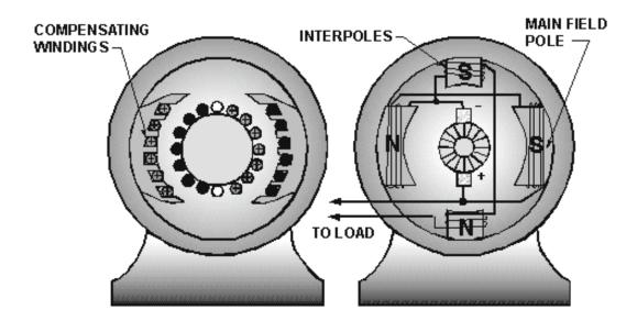
Figure 1-9.—Compensating windings and interpoles.
