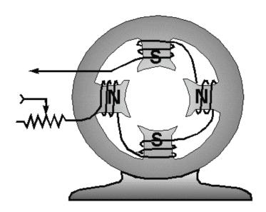
Figure 1-6.—Four-pole generator (without armature).
