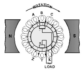
**ARMATURE REACTION** takes place when armature current causes the armature to become an electromagnet. The armature field disturbs the field from the pole pieces. This results in a shift of the neutral plane in the direction of rotation.
