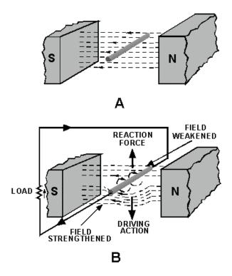
Figure 1-10.—Motor reaction in a generator.
