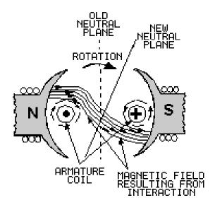
**COMPENSATING WINDINGS AND INTERPOLES** are used to counteract the effects of armature reaction. They are supplied by armature current and shift the neutral plane back to its original position.
