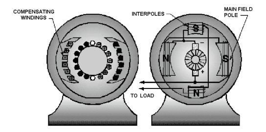
**MOTOR REACTION** is caused by the magnetic field that is set up in the armature. It tends to oppose the rotation of the armature, due to the attraction and repulsion forces between the armature field and the main field.
