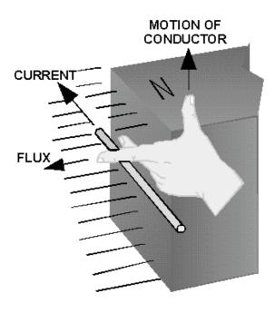
Figure 1-1.—Left-hand rule for generators.
