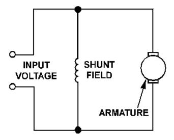
**ARMATURE REACTION** is the distortion of the main field in a motor by the armature field. This causes the neutral plane to be shifted in the direction opposite to that of armature rotation. Interpoles and compensating windings are used to reduce the effect of armature reaction on motor operation.
