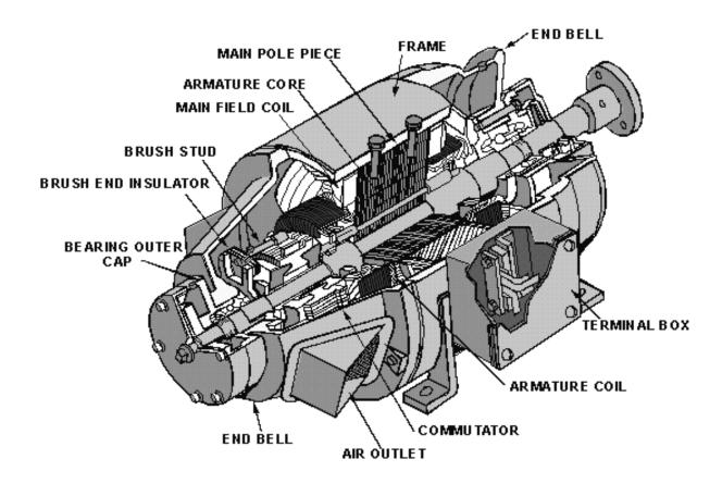
Figure 1-20.—Construction of a dc generator (cutaway drawing).
