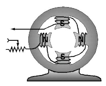
**COMMUTATION** is the process used to get direct current from a generator. The coil connections to the load must be reversed as the coil passes through the neutral plane. The brushes must be positioned so that commutation is accomplished without brush sparking.
