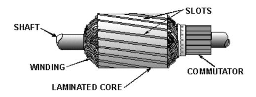
Figure 1-13.—Drum-type armature.
