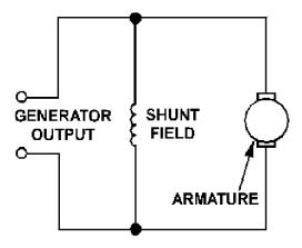
Figure 1-16.—Shunt-wound generator.
