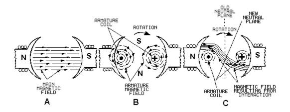
Figure 1-8.—Armature reaction.
