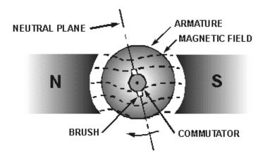
Figure 2-9.—Armature reaction.
