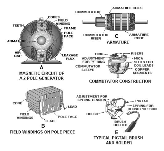
Figure 1-19.—Components of a dc generator.
