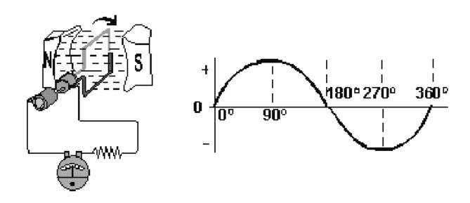
A **BASIC DC GENERATOR** results when you replace the slip rings of an elementary generator with a two-piece commutator, changing the output voltage to pulsating dc.
