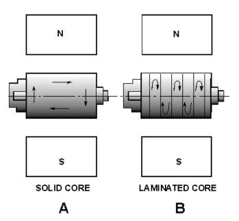
Figure 1-11.—Eddy currents in dc generator armature cores.
