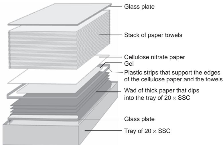
**Fig. 6.3.** Basic Blotting procedure
