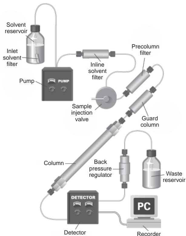
Fig. 4.6. HPLC Apparatus
