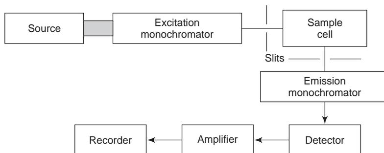
Fig. 11.2. A diagram of the arrangement of a Fluorimeter
