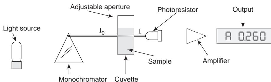
**Fig. 10.5.** An arrangement of colorimeter
