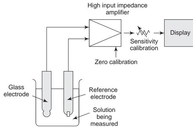
**Fig. 2.1.** The electrode system for measurement of pH
