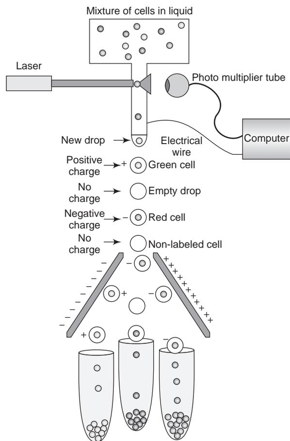
Fig. 11.3. Diagram showing cells population passing through Flow Cytometer
