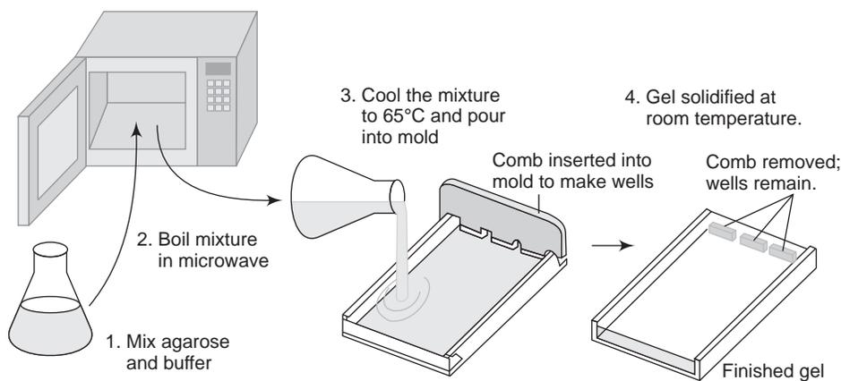
**Fig. 5.11.** Procedure of preparing the agarose gel
