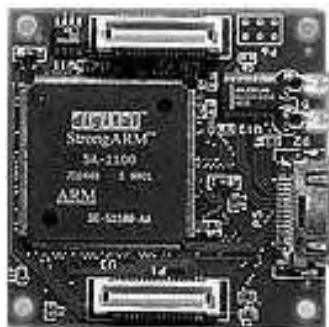
(a) The WINS processor board
