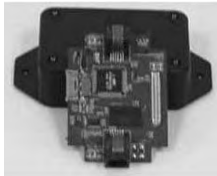
Fig. 2.14 Medusa MK-2 sensor node from UCLA.
