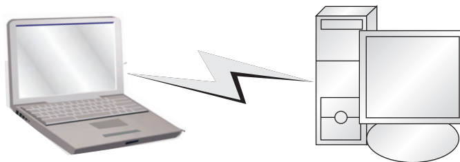
Figure 2.32(a): Peer-to-peer wireless LAN
