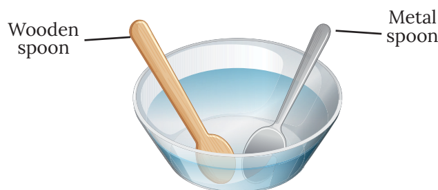
Fig. 4.16 Metal and wooden spoons immersed in hot water
