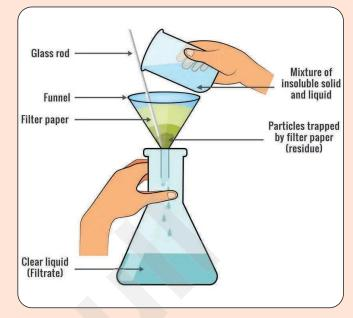
remains on the filter paper is known as the residue, while the clear liquid that passes through is called the filtrate. The filter paper thus acts as a sieve, allowing separation based on the particle size of the solid and liquid components.
