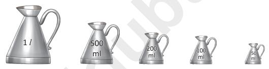
For measuring oil like petrol, diesel, kerosene etc.
