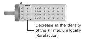
Right after the compression pulse, another pulse, called the rarefaction pulse, goes away from the piston just as fast as sound travels. This keeps repeating, and that's how the sound wave keeps moving forward.
