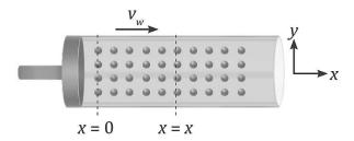
As sound travels through a substance, the particles in that substance move back and forth in a regular way, kind of like swinging in a straight line. This makes the position of the particles change in the following manner:
