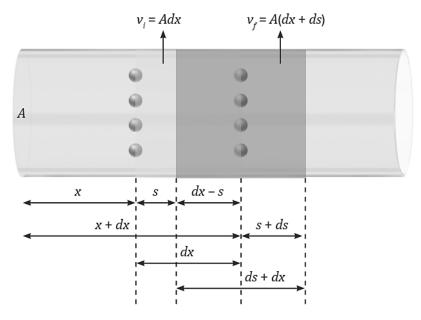
The volume enclosed between the two particles separated by a distance dx is given by,
