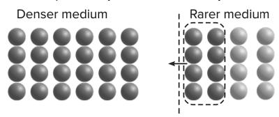
In simple terms, when a sound wave bounces off the thinner material, the squeezed part turns into a stretched-out part. So, we can say that the sound wave changes by half a circle  $(\pi)$  after bouncing off the thinner material.
