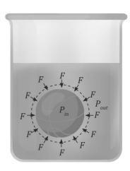
The bulk modulus is a measure of how a substance responds to pressure. It's significant when we're dealing with fluids like liquids and gases. The bulk modulus is always a positive number, and the negative sign in its formula shows that when the pressure goes up, the substance tends to get a bit smaller in response.
