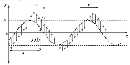
It is important to note that the velocity of the particle is a result of its SHM with respect to the equilibrium position, where y=0. In the x-direction, the particle's displacement is zero. The speed of the wave or disturbance that propagates in the x-direction is  $v\left(=\frac{\omega}{k}\right)$ .
