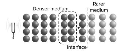
At this point, the place where they meet acts like a loose end (similar to how it works with string waves). Right after the collisions, the particles from the thicker material move into the thinner material and bounce back into the thicker one, but they bounce back as a stretch-out part. So, the thinner material (the loose end) acts like a point that moves a lot, as you can see in the picture.
