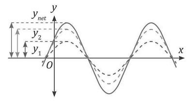
In this case, you can see that the highest point of one wave is matching up with the highest point of the other wave. And the lowest point of one wave is matching up with the lowest point of the other wave.
