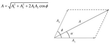
In this way, we can think of A as what you get when you combine two arrows,  $A_1$  and  $A_2$ , with an angle  $\emptyset$  between them. The size of the combined wave depends on how the two waves' timings match up or don't match up.
