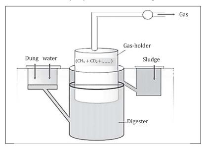
The organic wastes from the farm, including cow dung, urine, and feces, can be economically utilized to produce Gober gas, also known as biogas. Biogas typically consists of methane (50-70%), CO<sub>2</sub> (30-40%), and trace amounts of hydrogen, nitrogen, and hydrogen sulfide.
