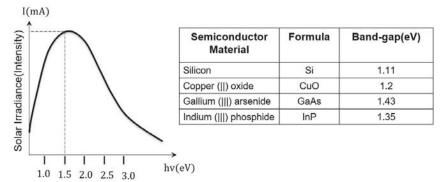
According to the graph, photons with energy close to  $1.5\ eV$  exhibit the highest intensity. Hence, materials selected for solar cell production typically possess a band gap ranging between  $1.0\ eV$  and  $1.8\ eV$ , as photons within this range demonstrate exceptionally high intensity.
