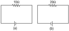
On the contrary, when the positive terminal of the battery is linked to point B, D2 is forward-biased, while D1 is reverse-biased. The equivalent circuit corresponding to this scenario is depicted in figure (b). The battery's current flow is calculated as 2 V divided by  $20 \Omega$ , yielding a current of 0.1A.
