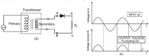
Since the output current corresponds to only one half of the input voltage wave, with the other half absent, this technique is known as half-wave rectification. The transformer's function in this process is to supply the necessary voltage to the rectifier.
