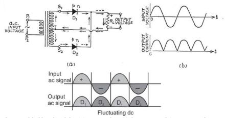
During the initial half-cycle of the AC input voltage, when terminal  $S_1$  is positively oriented with respect to T and  $S_2$  is negatively charged, junction diode  $D_1$  undergoes forward biasing, whereas  $D_2$  experiences reverse biasing. As a result,  $D_1$  conducts current, while  $D_2$  does not. The conventional current flows through diode  $D_1$ , the load RL, and the upper half of the secondary winding, as indicated by solid arrows.
