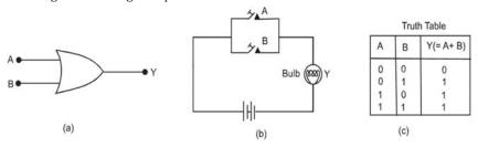
The myriad possible input combinations of A and B, alongside the resulting output Y of the OR gate, can be elucidated through the practical implementation of an electrical circuit, depicted in the accompanying diagram. This circuit comprises two switches, designated as A and B (representing the inputs), arranged in parallel to both a battery and a bulb Y (symbolizing the output).
