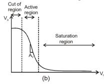
drive the transistor into saturation,  $V_0$  decreases nearly to zero. The transistor is deemed switched off when it's not conducting and switched on when driven into saturation. Therefore, establishing low and high states according to specific voltage levels corresponding to cut-off and saturation enables us to assert that a low input deactivates the transistor, while a high input activates it.
