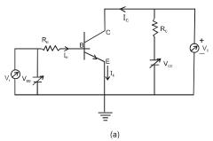
When  $V_i$  is below 0.6 V, indicating the cut-off state,  $V_0$  remains constant at  $V_{CC}$  with  $I_C$  being zero. As
