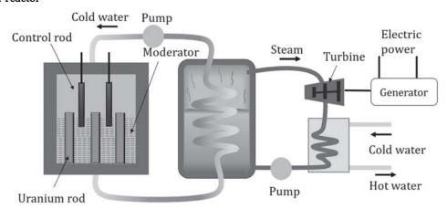
Within the reactor, the core serves as the location for nuclear fission, housing Uranium rods along with a moderator to decelerate neutrons. Encircling the core is a reflector, minimizing neutron leakage. Control rods, typically composed of cadmium, enable the reactor's shutdown by absorbing neutrons effectively. Heat generated during fission is extracted by circulating cold water, which in turn heats water within a tank, producing steam. This steam propels turbines, generating electricity.
