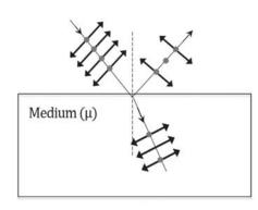
refracts, more vibrations happen parallel to that surface. Therefore, both the reflected and refracted light become partially polarized. Additionally, the amount of polarization in reflected light shifts as we change the angle of incidence i.
