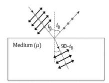
$$1 \times \sin i = \mu \times \sin r \xrightarrow[r=90^{\circ}-i_{B}]{} \sin i_{B} = \mu \cdot Sin(90 - i_{B}) \Rightarrow \tan i_{B} = \mu$$
