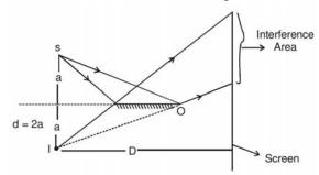
A significant aspect of this experiment is that when the screen touches the end of the mirror, the edge of the mirror's reflecting surface falls at the center of a dark fringe instead of a bright one. The direct beam doesn't experience any phase change, indicating that the reflected beam undergoes a phase change of  $\pi$  radians.
