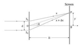
$$\begin{split} \Delta x &= \lambda/2 = 1^{st} \text{ Minima} \\ \Delta x &= 3\lambda/2 = 2^{nd} \text{ Minima}. \\ &\vdots \\ \Delta x &= (2n-1)\lambda/2 = n^{th} \text{ minima} \end{split}$$
