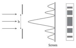
In YDSE, all the maxima have the same intensity whereas in case of Fraunhofer diffraction, the intensity of maxima decreases as we move away from the central maxima.
