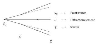
When light passes through a pinhole or a narrow slit, we notice a bright spot in the center of the screen. The size of this spot is larger than the size of the pinhole or slit. Additionally, we see dark and bright rings encircling the central bright spot.
