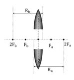
Cutting of a lens perpendicular to the principal axis.
