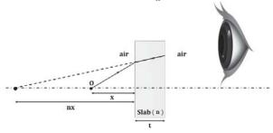
Hence, the distance between the object and the position of the image is altered due to the presence of the slab.
