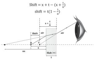
Since the shift is not influenced by the position of the object (x), the same displacement will be observed regardless of where the object is located.
