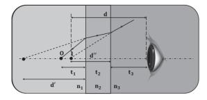
Shift from a slab; Object and Observer are in different mediums (n mediums)
