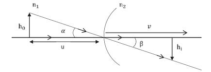
$$Magnification = \frac{\frac{\text{Height of image}}{\text{Height of object}}}$$
