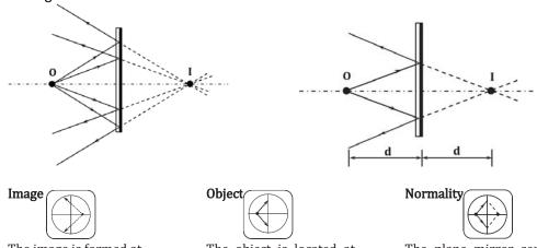
The image is formed at the point where the reflected rays intersect. The object is located at the point where the incident rays intersect.
