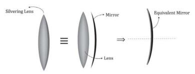
Upon incidence on the silvered lens, the incident ray reflects back to incident medium. Therefore, the equivalent system will be a mirror.
