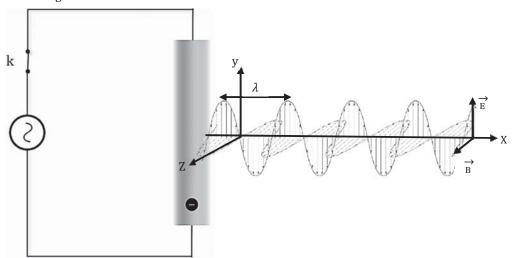
The oscillations of electric and magnetic fields mutually regenerate, initiating the propagation of electromagnetic energy through space, forming what is known as an electromagnetic wave. The energy linked to the advancing wave is obtained at the cost of the energy from the source.
