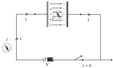
Ampere's Law as applied to the needle positioned at point 1:  $\oint B \cdot dl = \mu_0 i_0$
