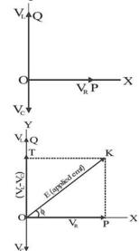
Finally, the vector OK represents the resultant of  $V_R$  and  $(V_L - V_C)$ , that is, the resultant of all the three = applied e.m.f.
