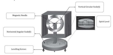
When we adjust the setup using leveling screws and a spirit level, it's possible that the magnetic needle isn't aligned with the Earth's magnetic field direction, known as the magnetic meridian. The needle's orientation might deviate from the magnetic meridian by an angle  $\beta$ , as depicted in the diagram. Consequently, the Earth's magnetic field ( $B_e$ ) differs in these two orientations.
