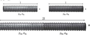
The rods are joined in such a way that the resistance of resulting material i.e., the equivalent resistance of the configuration doesn't vary with temperature. Therefore, the equivalent resistance of the rods before and after an increase of temperature should be same.
