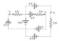
If we go from negative terminal of the battery to the positive terminal of the battery, then potential at the positive terminal = (potential of the negative terminal + potential difference of the battery) Therefore,
