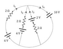
The potential difference across the 2  $\Omega$  resistance connected between point C and G is, [6-(-10)]=16V Therefore, the current through it from C to  $G:i_1=\frac{16}{2}=8A$  [Since C has higher potential than G, the current will flow from C to G]
