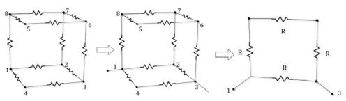
Equivalent resistance of the top and bottom part of the circuit: R
