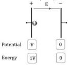
The energy expended to transport a unit positive charge from a lower potential to a higher potential is termed as EMF (Electromotive Force).
