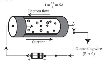
Suppose the current in the circuit is created by the motion of positive charge carriers, represented by  $e^+$  or positrons.
