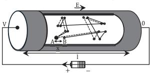
With battery connected, the motion of the charge carriers will remain random but there will be some effective displacement. Thus, the following results are observed:
