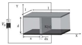
In this context, the dielectric constant K changes along the y-axis. Let's consider a small strip of dielectric material located at a distance y from one of the plates, with a thickness dy. The entire dielectric slab consists of several such strips connected in series. If the length of each strip is l, its cross-sectional area is  $l^2$ .
