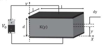
The capacitance associated with a small strip,  $dc = \frac{g_0 k(y) l^2}{dy}$ .
