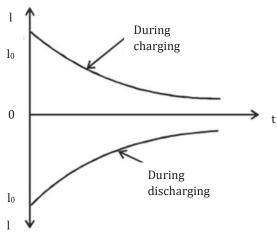
$$I = I_0[e^{-(RC/RC)} = \frac{I_0}{e} = 0.37I_0 = 37\% \text{ of } I_0$$
