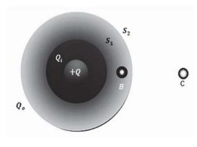
For cavities with arbitrary shapes,  $Q_i$  is distributed non-uniformly across the inner surface. However, it's arranged in a manner that ensures the electric field outside the cavity's surface, caused by the total charge within the cavity (i.e.,  $Q_i + Q$ ), remains zero.
