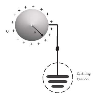
$$\begin{split} \frac{k(\theta-q)}{R} &= \frac{kq}{R_e} \\ \theta-q &= \frac{Rq}{R_e} \\ \theta &= q[\frac{R+R_e}{R_e}] \\ q &= [\frac{\theta R_e}{R+R_e}] = \frac{\theta}{1+R_1/e_e} \end{split}$$
