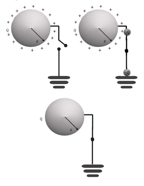
In this scenario, a positive charge +Q is positioned adjacent to an initially uncharged isolated conductor. Consequently, the system no longer remains isolated. When the conductor establishes a connection with the Earth, its potential tends toward zero. Let q' represent the charge that flows from the Earth to the conductor.
