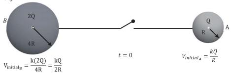
At time t = 0, when the conductors are not connected, the voltage at point B is lower than the voltage at point A.
