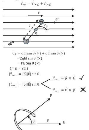
Torque operates with the intention of orienting the dipole in alignment with the electric field's direction.
