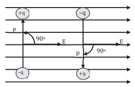
The magnitude of the torque reaches its peak when the dipole is positioned perpendicular to the direction of the electric field.
