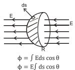
Where  $\int$  ds cos  $\theta$  is Projection of the spherical surface Area on base.
