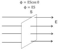
**Case II:** If electric field is parallel of the surface (glazing), then angle made by  $\vec{E}$  with normal=90°
