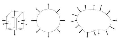
For closed surfaces, the area vector's direction is invariably perpendicular to the surface, with the normal directed outward.
