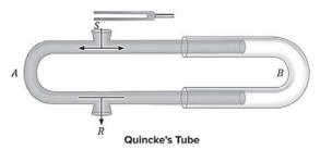
Tube A is equipped with two openings: (i) S, serving as the source generating sound waves, and (ii) R, designated as the receiver or detector. The sound waves generated by the source split within tube A, and the resulting two beams of sound waves combine at the receiver. Due to their common origin, these two beams are coherent. Consequently, interference occurs at the receiver or detector. The overall phase difference between these two sound wave beams is then determined by.
