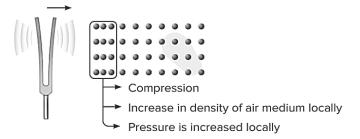
Following the creation of the compression pulse, the prong then reverses its motion, moving inward. This action pulls away some air from the area in front of it, resulting in a slight decrease in pressure below the average. This diminished pressure region is identified as a rarefaction pulse.
