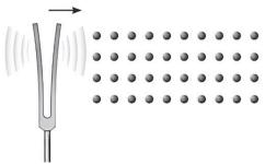
The area of heightened pressure is referred to as a compression pulse, and it propagates away from the prong at the speed of sound.
