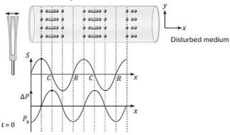
The term "excess pressure" ( $\Delta P$ ) indicates that the pressure at a specific point exceeds the average pressure ( $P_0$ ) of the medium.
