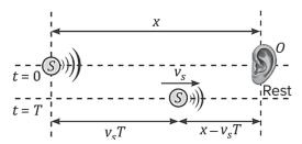
Assuming the velocity of the sound wave in the medium is v, the observer receives the first pulse after  $T_1 = \frac{x}{v}$  time. As the second pulse is emitted from the source after a time interval T from the first one, and at that moment, the source is at a distance of  $(x - v_s T)$  from the observer, the time for the second pulse to reach the observer can be expressed as:
