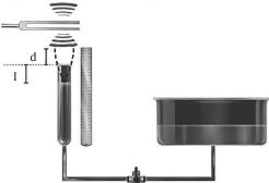
If the length of the air column for the first resonance is  $l_1$  and the end correction is d, then the condition for the first resonance to occur is,
