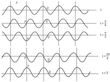
Upon close examination of the image, it can be observed that particles P and Q return to their initial positions after one time period T. Consequently, one can infer that each particle on the string undergoes Simple Harmonic Motion (SHM) with the same amplitude and time period as the source. In summary, every particle on the string wave exhibits identical characteristics to those of the source. Thus, the wave equation reflects the equation of the source undergoing SHM.
