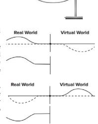
Hence, it can similarly be deduced that the shape of the pulse during reflection can be determined by overlaying the inverted pulse onto the incident pulse.
