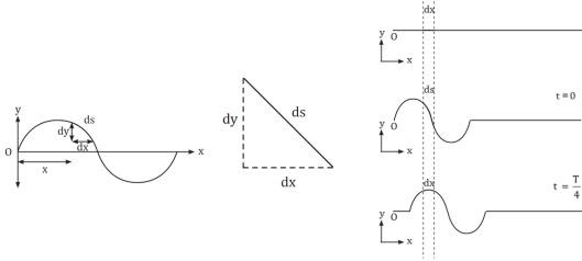
The work done by the tension force, dU = F(ds - dx) (Since (ds - dx) is the displacement) Here, the only force acting is tension (T). Therefore,
