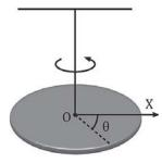
Therefore, the elongated body undergoes torsional oscillations with angular frequency,  $\omega = \frac{c}{\sqrt{L}}$
