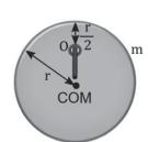
Sol. (a) The moment of inertia of the ring about the COM is, I COM =  $mr^2$ . Thus, the moment of inertia of the ring about point O is,  $I = I_{COM} + mr^2 = mr^2 + mr^2 = 2mr^2$
