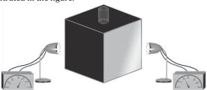
This experiment confirms that black color serves as both an effective absorber and emitter of heat. Consequently, materials that excel at absorbing heat also excel at emitting it. This principle holds true for all substances.
