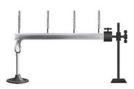
This creates a temperature gradient along the length of the rod. Moving from left to right, the temperature of the rod decreases, as indicated by the thermometers. The temperature gradient continues to fluctuate until it stabilizes at a steady state. At this point, the amount of heat crossing any cross-section of the slab per unit time becomes equal. Consequently, the rate of heat flow remains constant over time.
