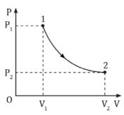
Therefore, we can infer that the gas will perform work, which reduces its internal energy. As a result of this decrease in internal energy, the gas's temperature will also decrease ( $T_2 < T_1$ ). In an adiabatic compression ( $\Delta Q = 0$  and  $V_2 < V_1$ ), the work is done on the gas by the surroundings. Thus,
