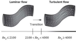
If the Reynolds number is less than or equal to 2100, then the flow comes under the laminar flow. If it is between 2100 and 4000, then the flow comes under the transition flow. For turbulent flow, the Reynolds number is greater than or equal to 4000.
